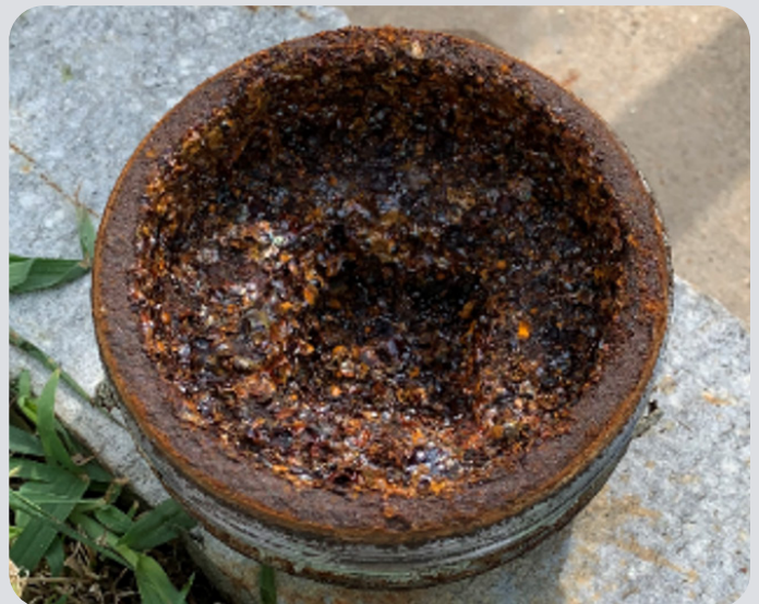
Corrosion on Underside of Bung
