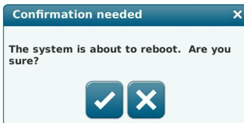
15. Wait for the console to automatically cycle power. When it starts back up, verify the new software version. Go back to the **Activate/Revert** screen and the new software version will be displayed next to **Available Version**.
