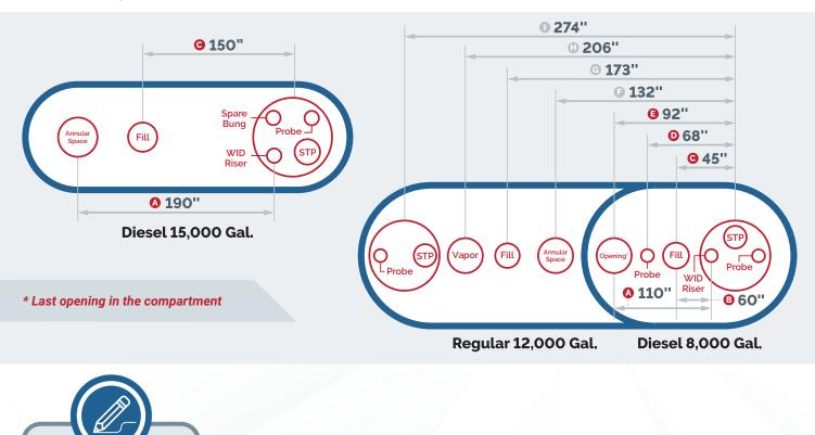
Use the tank outline on the right to draw in your tank configuration details with measurements like the examples above
