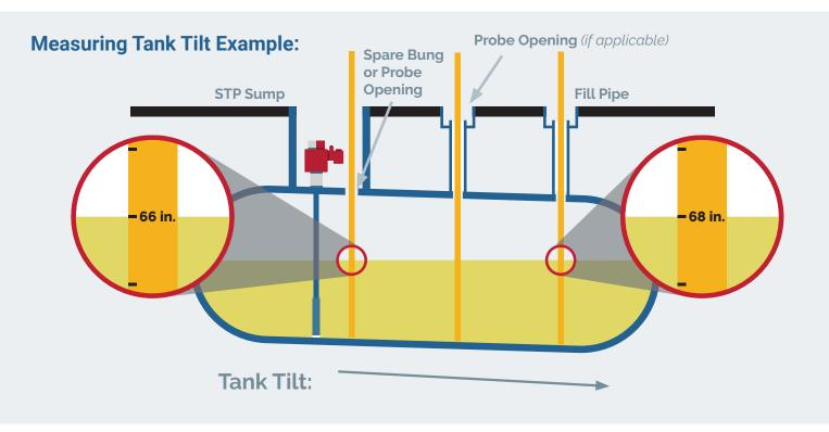
Stick the tank at the **Probe Opening** in the **STP Sump**, at the **Fill Pipe**, and at the separate **Probe Opening** (*if applicable*) to determine tank tilt. Place the stick heights on the tank diagram below next to each location. Please be as precise as possible.
