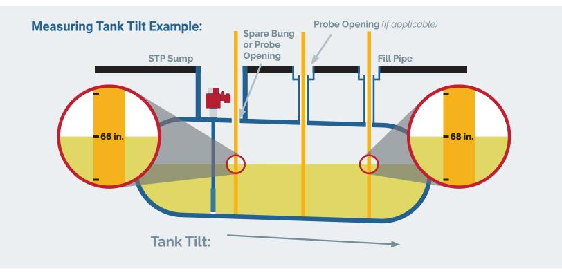
Stick the tank at the **Probe Opening** in the **STP Sump**, at the **Fill Pipe**, and at the separate **Probe Opening** (*if applicable*) to determine tank tilt. Place the stick heights on the tank diagram below next to each location. Please be as precise as possible.
