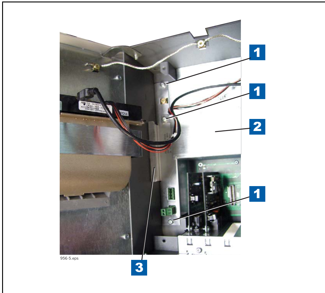
Figure 7-9. Removing AC Input Filter
