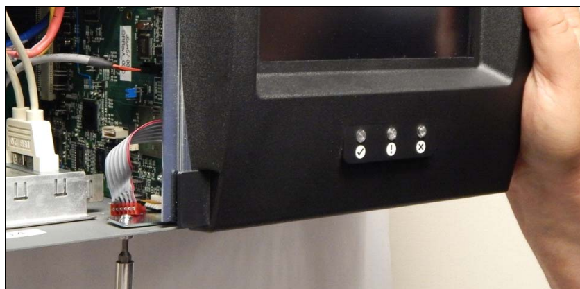
Figure 7-5. Remove Top And Bottom Optional Display Door Hinge Screws
