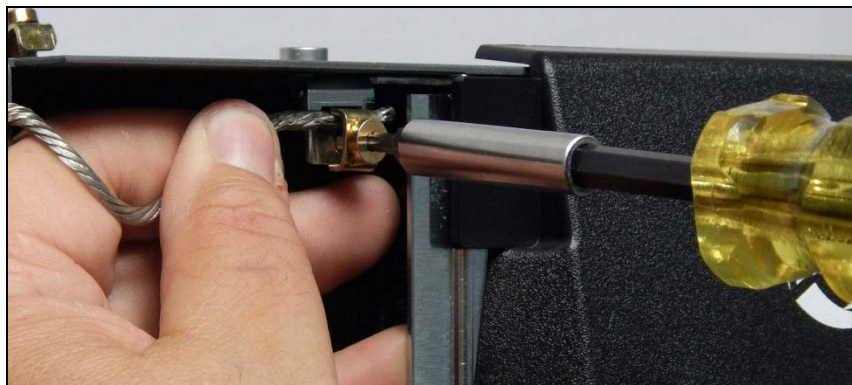
Figure 7-4. Remove Ground Wire From Ack Switch/Display Door
