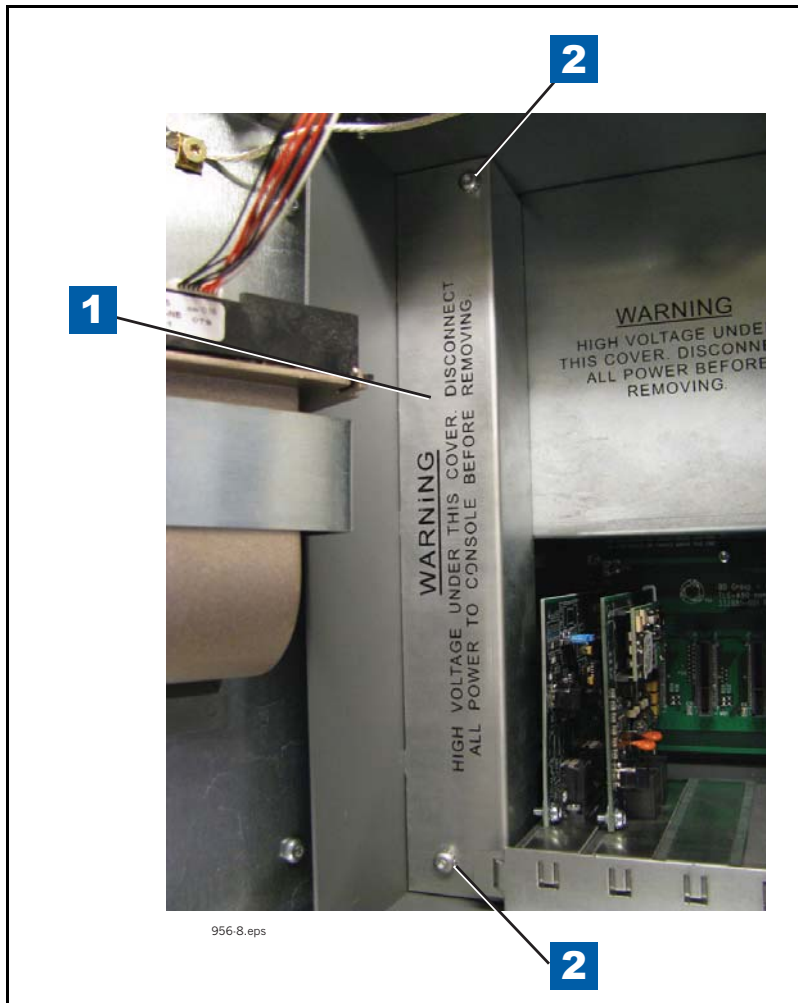
Figure 7-8. Remove AC Channel Cover
