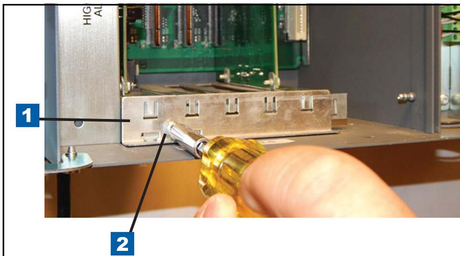
Figure 10. Removing Comm Module Clamp
