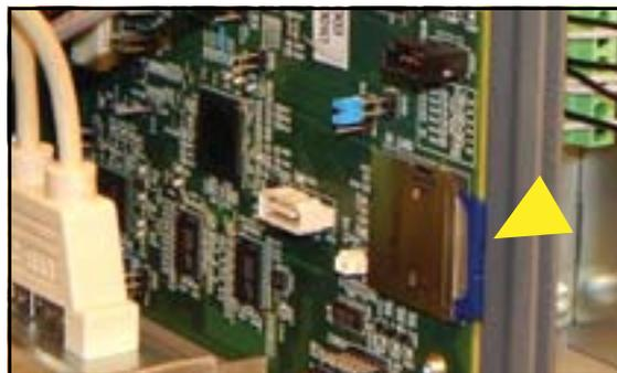
Figure 24. Locating SD Card On CPU Board
