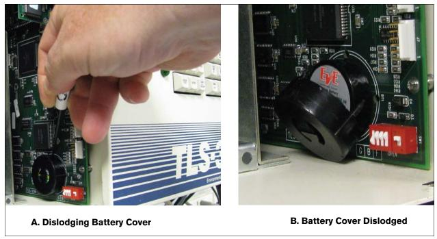
Figure 2-14. Removing Battery Cover
