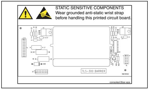
Figure 2-10.TLS-300 Series Console I.S. Barrier Board
