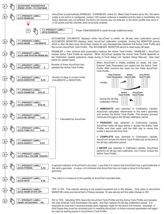
Figure 6-10. **AccuChart Diagnostic Function Diagram**
