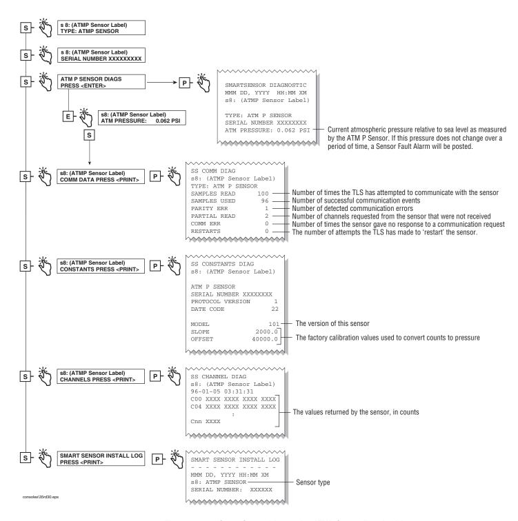
Figure 6-32. Smart Sensor Diagnostic - ATMP Sensor Function Diagram
