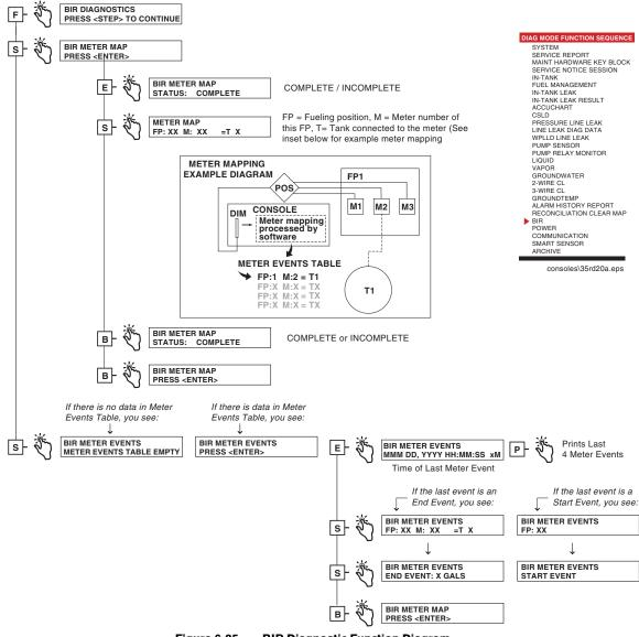
Figure 6-25. BIR Diagnostic Function Diagram
