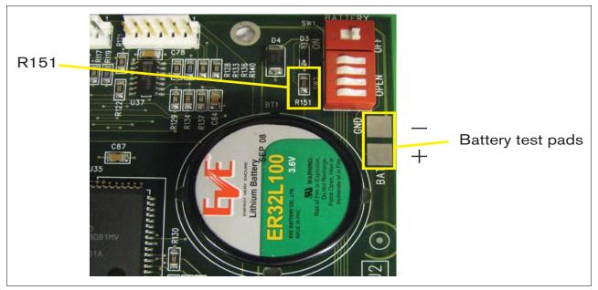
Figure 2-13. Battery Voltage Test Locations On ECPU Board
