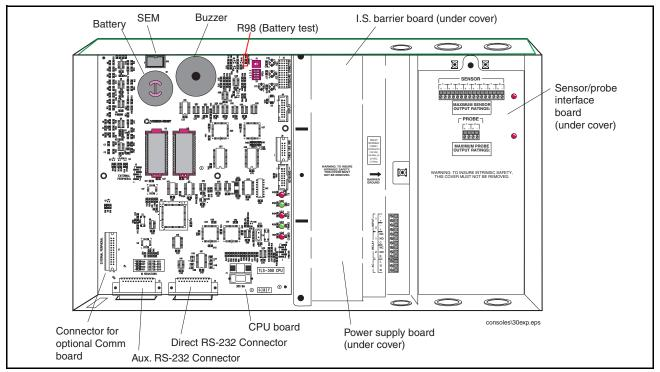
Figure 2-3.PC Board Identification (TLS-300 Series Consoles Shown With Doors Removed)
