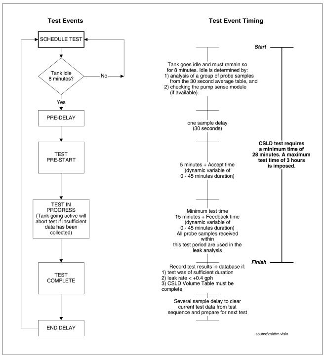
Figure 11-2. CSLD Leak Test Timing Sequence
