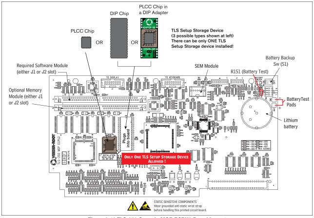
Figure 2-12.TLS-350 Console MSP ECPU2 Board Layout
