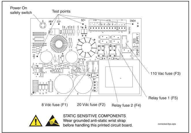
Figure 2-9.TLS-300 Series Console Power Supply Board
