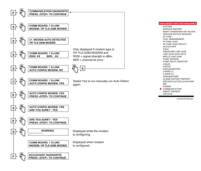
Figure 6-27. Communication Diagnostic Function Diagram
