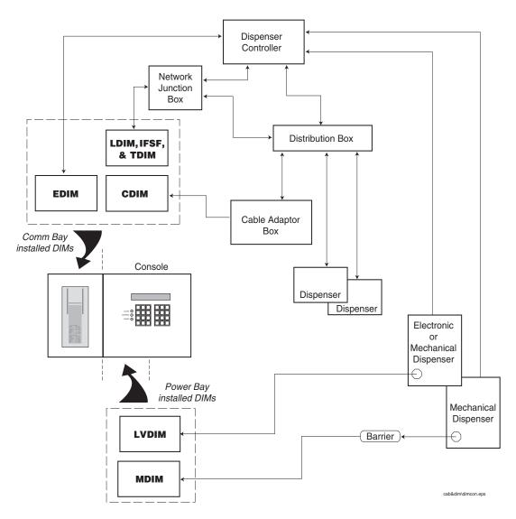
Figure 10-1. Simplified DIM Connections To Various Dispensing Systems
