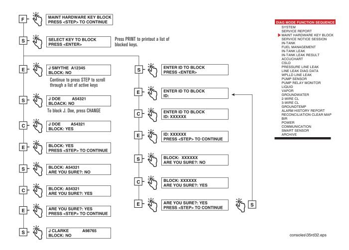
Figure 6-4. Maintenance Hardware Key Block Function Diagram
