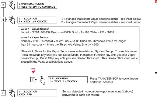
Figure 6-18. Vapor Sensor Diagnostic Function Diagram
