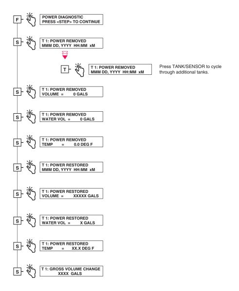
Figure 6-26. **Power Diagnostic Function Diagram**
