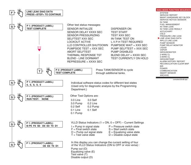
Figure 6-13. VLLD Diagnostic Function Diagram
