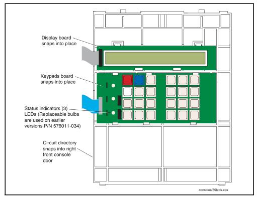
Figure 2-4. Console Display/Keyboard Board Components (Behind Right Door)
