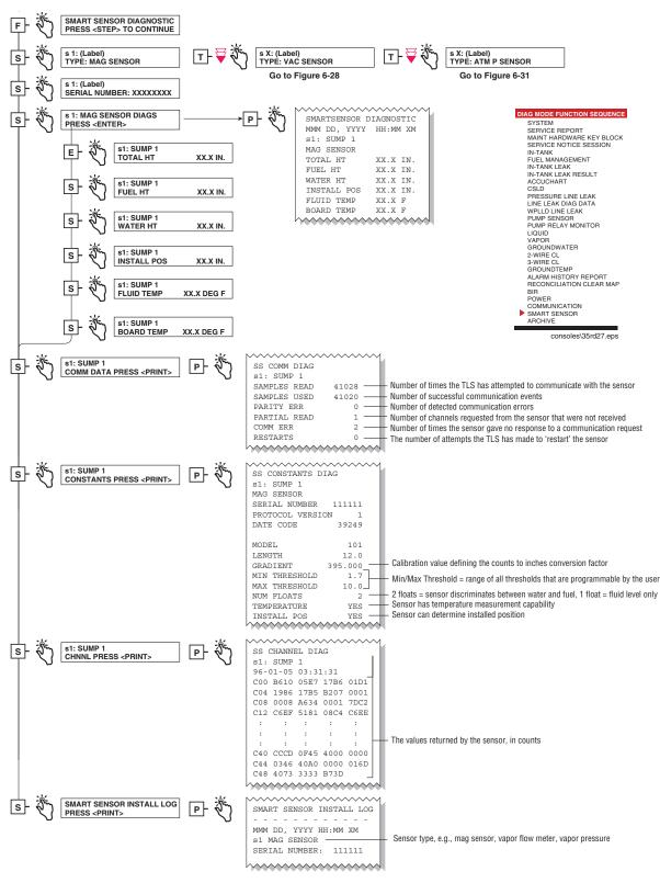
Figure 6-28. Smart Sensor Diagnostic - Mag Sensor Function Diagram
