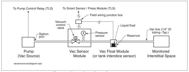
Figure 8-1. Vacuum Sensor System Components
