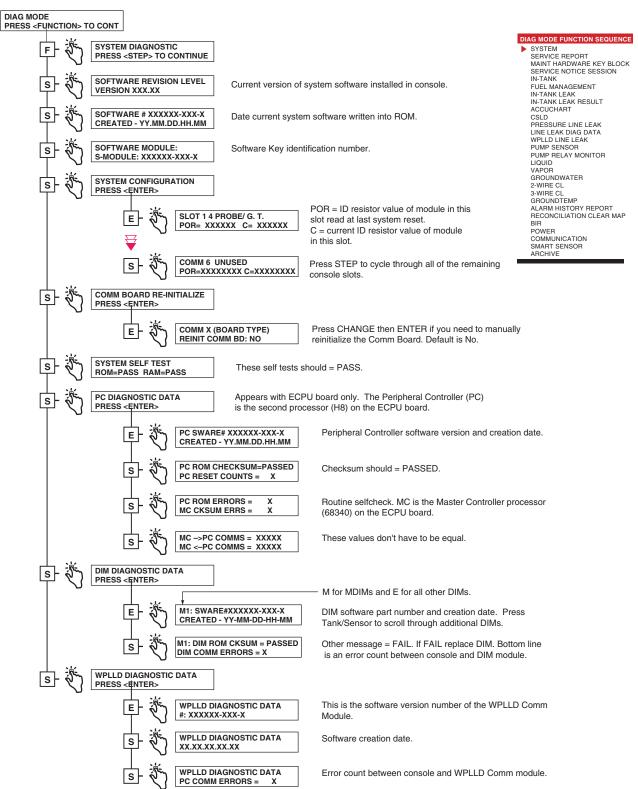
Figure 6-2. System Diagnostic Function Diagram
