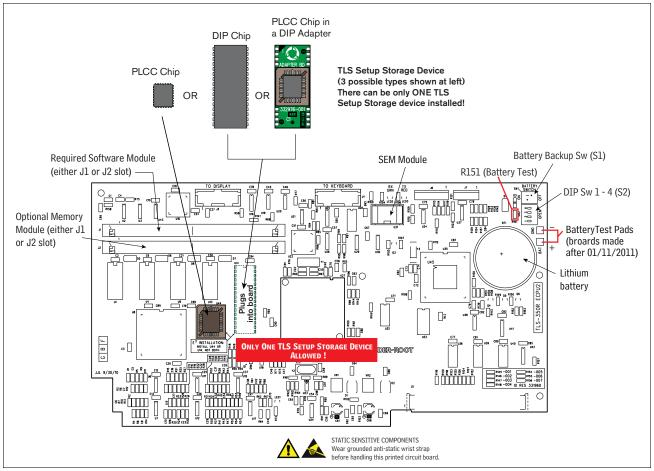
Figure 2-5. TLS-350 Consoles ECPU2 Board Layout
