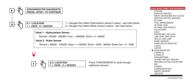
Figure 6-19. Groundwater Sensor Diagnostic Function Diagram
