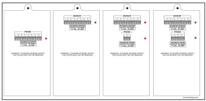
Figure 2-11.Example TLS-300 Series Console Sensor/Probe Interface Boards (8P/0S, 8S/0P, 8S/2P, And 8S/4P)
