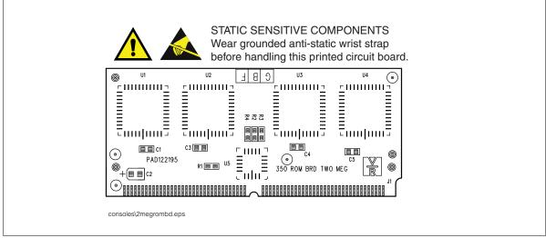
Figure 2-6.TLS-350 Series Console - 2 Meg ROM Board
