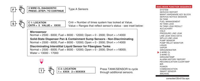
Figure 6-20. 2-Wire CL Sensors Diagnostic Function Diagram
