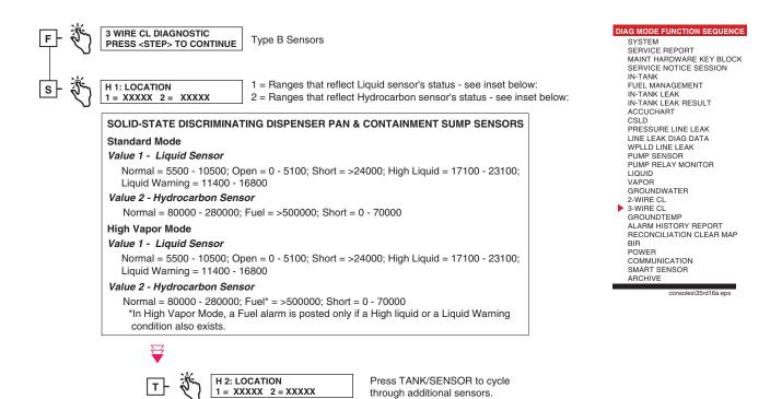
Figure 6-21. 3-Wire CL Sensors Diagnostic Function Diagram
