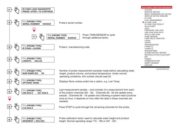
Figure 6-8. In-Tank Leak Diagnostic Function Diagram
