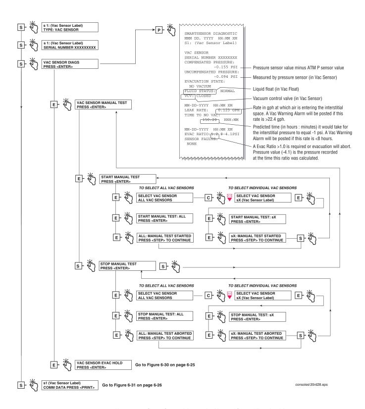
Figure 6-29. Smart Sensor Diagnostic - Vacuum Sensor Function Diagram
