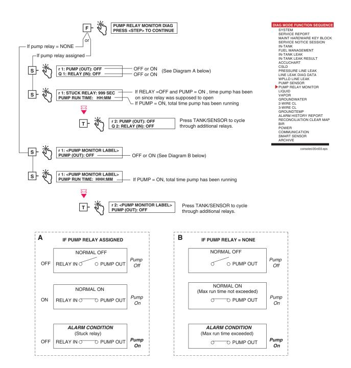
Figure 6-16. Pump Relay Monitor Diagnostic Function Diagram
