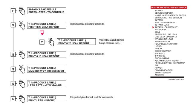
Figure 6-9. In-Tank Leak Result Diagnostic Function Diagram
