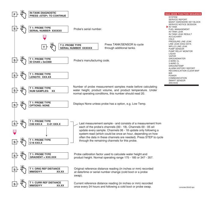
Figure 6-6. In-Tank Diagnostic Function Diagram
